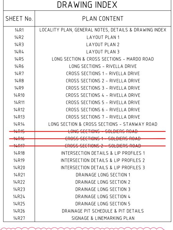
SHEETS 15, 16 AND 17 HAVE BEEN REMOVED FROM HONOUR VILLAGE STAGE 14 CONSTRUCTION DRAWING SET. THE INTERSECTION OF SOLDIERS ROAD AND RIVELLA DRIVE WILL BE CONSTRUCTED AS PART OF FUTURE STAGE 18 WORKS
