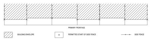
All side and rear fences are to be constructed of timber palings with a timber cap across the top, exposed timber posts on both sides of the fence, and to a height between 1.8 and 2.0 metres, including capping (excluding a screen required for overlooking purposes).
