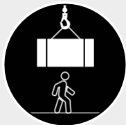
Person(s) being struck by dropped loads or between loads
