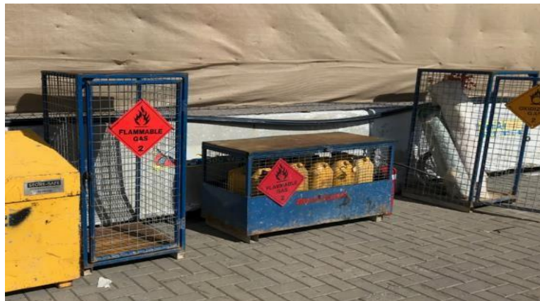
Figure 4.7.6.1.2– Spare Fuel Contained in Bunded Flammable Cages
