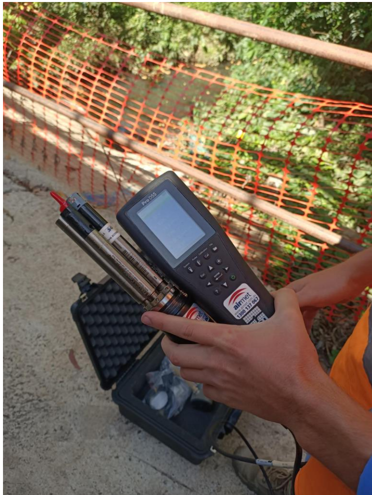
pH and turbidity testing device
