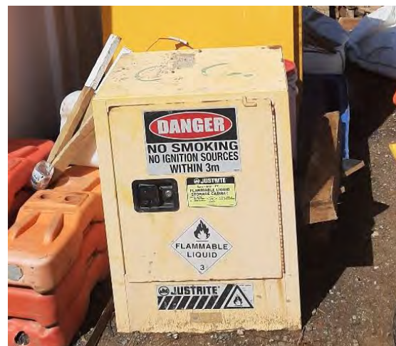
26. Secure storage for flammable liquid.
