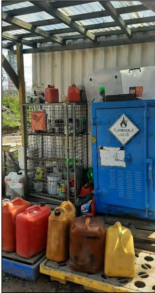
23. Unlocked cage storage for chemicals. Empty containers outside of cage.
