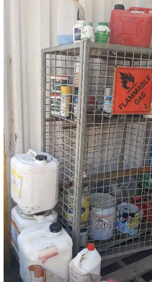
24. Containers inside and outside unlocked cage.
