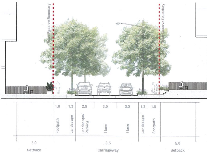
Figure 21 Cross section of the Neighbourhood Street typology
