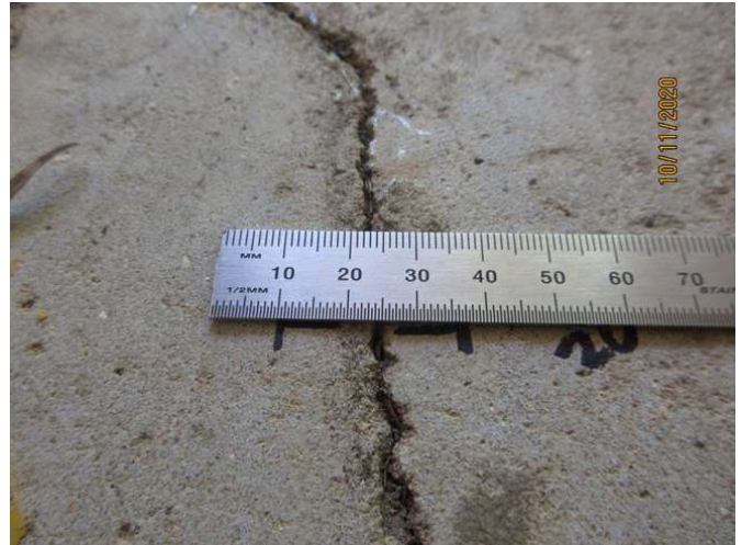
No 1-3_452_Note an estimated 1.5mm cracking width at representative location
