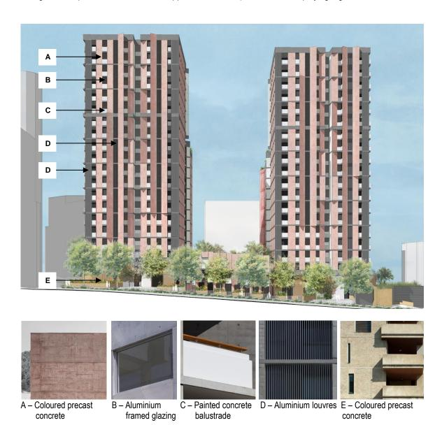
Figure 26 – South-West elevation material palette
