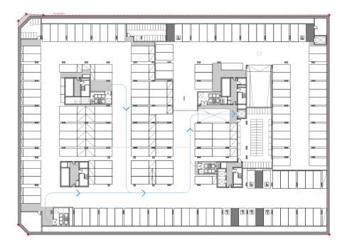
Figure 12.1 – Basement Level 3 plan showing waste strategy
