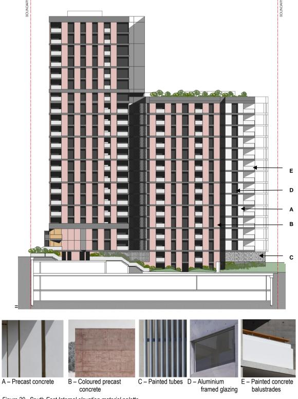
Figure 29- South-East Internal elevation material palette
