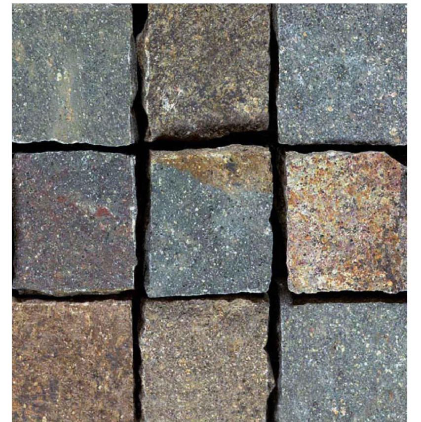
BASALT PORPHYRY STONE (90X90mm WITH 10-15mm MORTAR GAP)
