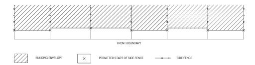
All side and rear fences are to be constructed of timber palings. A timber cap is to go across the top to a height between 1.8 and 2.0 metres including capping (excluding a screen required for overlooking purposes).
