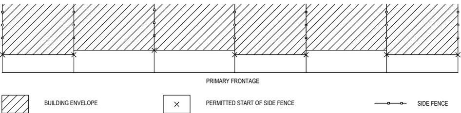
All side and rear fences are to be constructed of timber palings with a timber cap across the top to a height between 1.8 and 2.0 metres, including capping (excluding a screen required for overlooking purposes).
